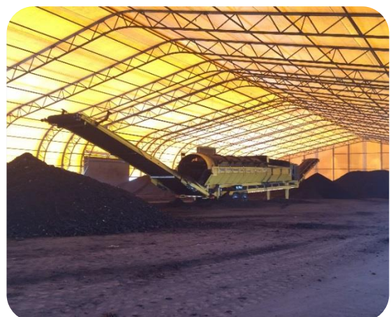
Screening SoilPro with a portable trommel screen in the storage facility
