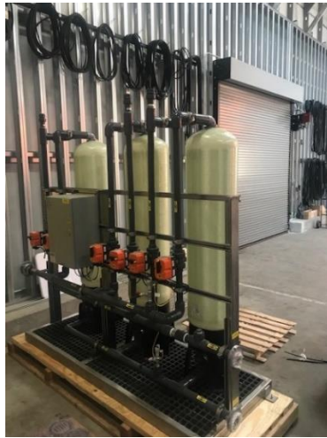
Automated water filtration system with backwash to drain
