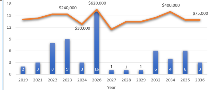
RP-1 # of VFD Replacements and Cost based on 15-Year Life Span by Year
