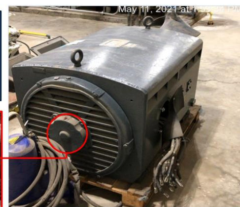
Pallet storage, no isolation from transient vibration
