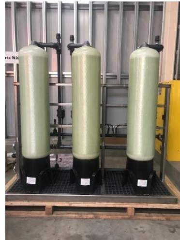
Automated water filtration system with backwash to drain
